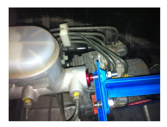
Finally make sure the red washer is pushed up against the master cylinder and can't rattle around.
