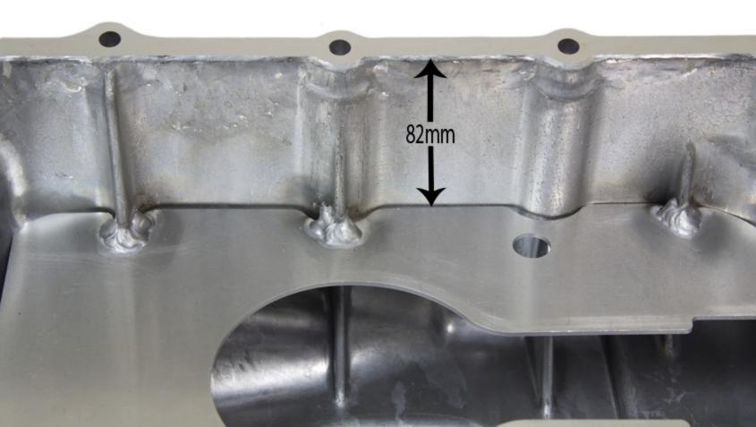
The plate needs welding so that the top face is 82mm from the machined face of the sump
