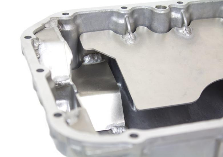
The plate needs welding so that the top face is 82mm from the machined face of the sump
