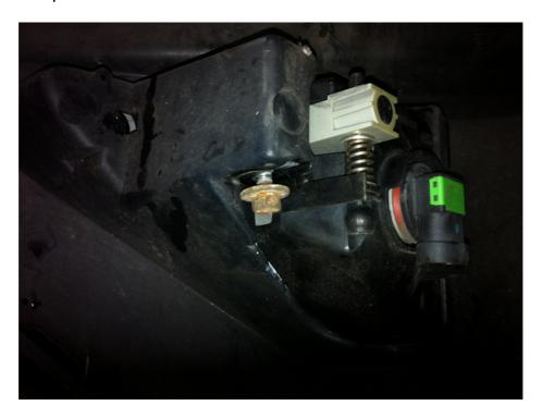
• Fit the fog scoops into the holes using the 10mm bolts, nuts and washer supplied. Make sure they are tight into the bumper before you tighten the bolt.
