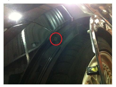
• Undo this screw, and repeat the other side. Next go under the car and remove the bolts and clips under the bumper. Again, here is a picture of it off the car to make it easier to show:
