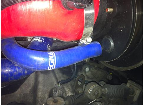
Fit the original induction hose back into the car and secure with the jubilee clips.
