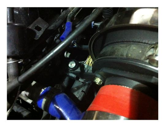
Now fit the breather hose. The short side of the right angle bend goes onto the cam cover, and the other
