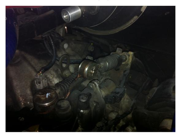
• Refit the gear cable clips and your air intake. Make sure everything is tight and test your gear shift action.
