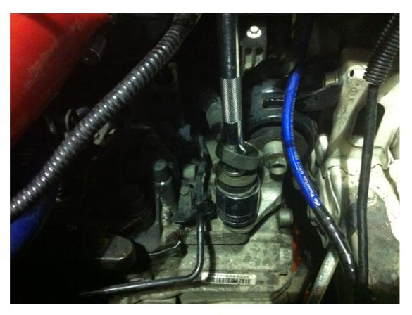
• Use some grease on the shifter bushes. We used copper grease but moly grease would be better. Slot one half of the bushes onto the gearbox first, followed by the cable, then the other half of the bush.
