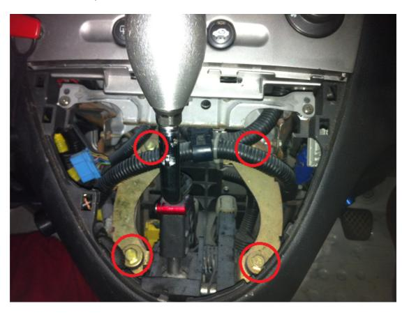
Remove these four 12mm bolts and push out the bushes. Push the
