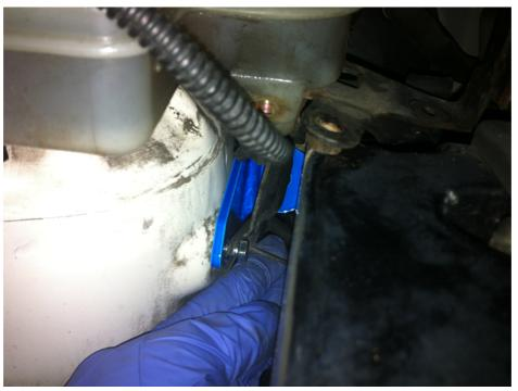
• At this point while the bracket is loose it is easier to refit the brake reservoir, hook it through now and bolt it back on.
