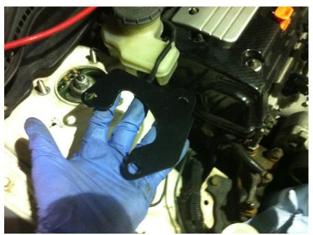
• Remove the 17mm nut nearest the front of the car on the right hand side engine mount, then place the other ETD bracket onto the studs. Refit the original nut and fit the supplied nut onto the rear bolt.
