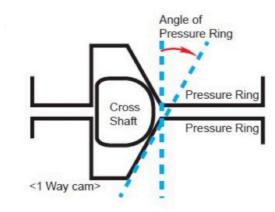
Initial preload is around 85lb. To change the preload, you need to remove or add springs, (there must be equal numbers i.e. 4, 6, 8, 10, 12). Unfortunately, the only way to check the preload value is to use a torque wrench with a special tool that is inserted into the LSD (like an axle shaft). The more preload you have set the quicker the onset of lock. (6 springs will provide approximately 55lbs)
