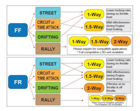
To change the "way" of the LSD for example from a 1.0 to a 1.5 you have to open the LSD. To do this remove the shipping screws and pull the two sections apart. Once open revolve the cam/adaptor to the position shown in the diagram below. The cross-pin needs to have the rounded part pointing the opposite way to the diffs
