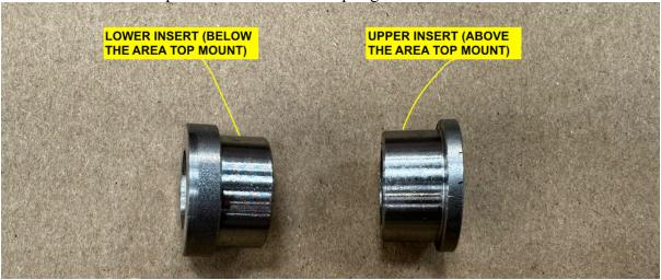
5. The lower insert measures 5.1mm and the upper measures 2.6mm.
