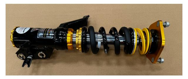
1. Disassemble the YSR by removing the 21mm (M14) nut on the top of the damper.
