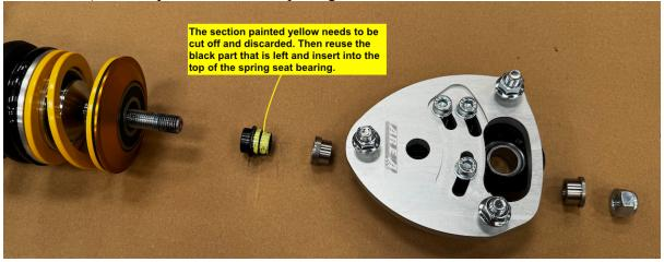
4. Please note that the top hat inserts <u>MUST</u> be installed the correct way around otherwise the top mount will rub on the spring carrier/seat.
