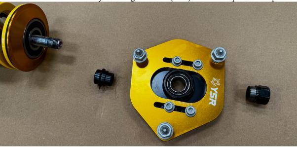
2. If you have an older set of dampers with M12 top nuts the setup will look slightly different, and the spring top seat will also be different. To fit the Area Top Mount the components should be put together in this order.
